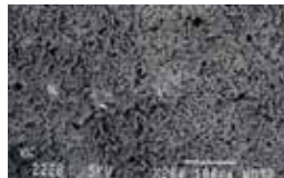
SEM PLGA magnification: 200X
